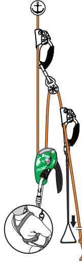
Example: Operator climbing a rope with control rope passed through Pulley on a hand ascender and second ascender and foot loop on the tail rope.
