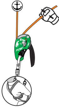
Example: Climber Pulling rope up through FLOW whilst simultaneously standing in foot loop.
