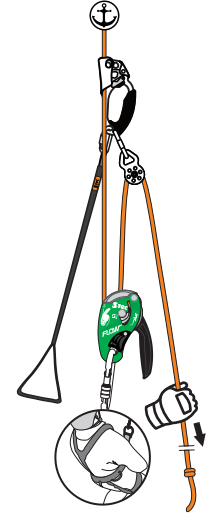
Example: Operator climbing a rope with control rope passed through Pulley on a hand ascender.
